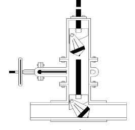
Hot tap on line previously made, line stopper attached to temporary valve and valve opened. Line stopper hydraulically or mechanically pushed into line to seal the pipe.
