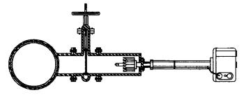
A. Saddle or weld nozzle installed, valve installed, assembly pressure tested and tapping machine attached.
