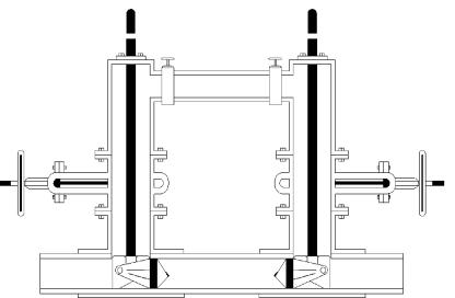
Two or more line stops can be used in conjunction to isolate and bypass many intersecting lines at once.
